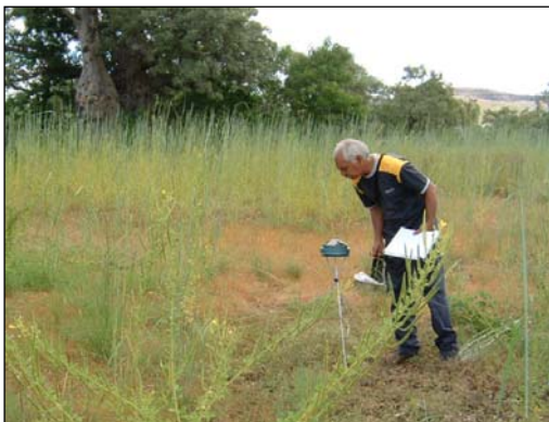
Bushlight's David D'Antoine checking the solar pathfinder at a proposed array site, Dingo Spring.
