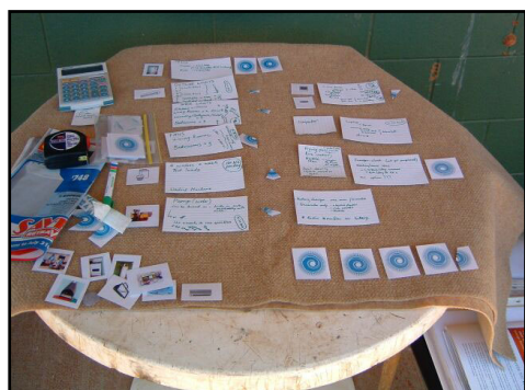
The final energy budget for the Green House at Mt Peachy. The blue energy icons at the bottom right of the photo show the daily system capacity required to run the fridge, lights, fans, washing machine, TV and video, computer and a Playstation. We also allowed enough for a freezer, which the household want to buy soon.
