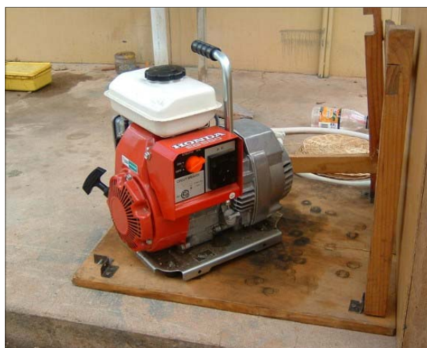
Honda 2.5kVA portable generator used for electrical power
