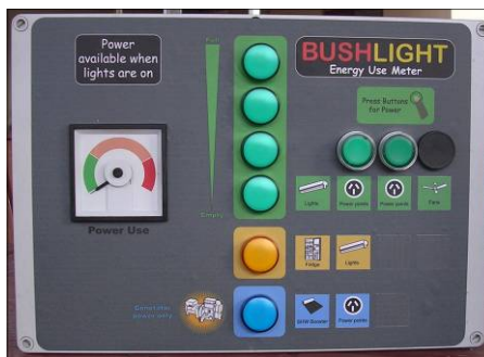
Bushlight Energy Management Unit
